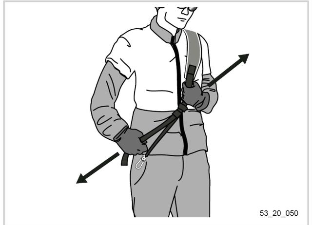
3. Pass the self-attaching fastener end of the strap under the main carrying strap.
