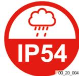
IP54 protection rating of the tool (allow protection against dust and water spray).
